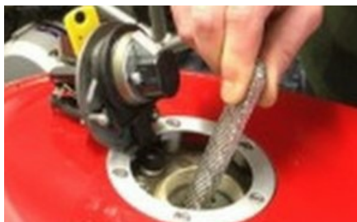
A fuel catalyst tank unit being fitted into a motorcycle fuel tank
